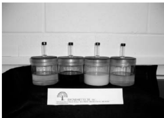
Figure 5: Several different antifouling paints prepared from PAMAMOS dendrimers and HB-PUSOX. Note that because the base polymer solutions are colorless, different colors originate from different antifoulants used. Small vials on the tops of the respective paint containers contain catalyst solutions that may or may not be needed (see text for explanation). (see page 4 of color insert)
