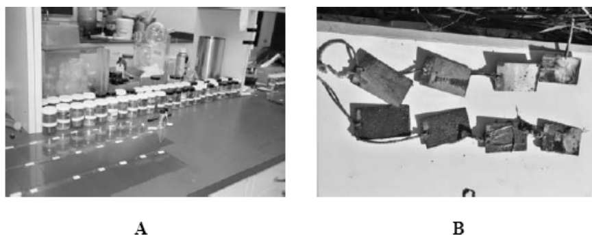
Figure 6: Testing of PAMAMOS-based antifouling paints. (A) Sample preparation: steel plates (lower left corner) ready for testing in Sanford Lake, MI; vials with samples submerged in the same lake water (upper center and right) for leaching tests. (B) Test plates from A after 3 months in Sanford Lake (according to Reference 32): notice small specks on the lower row of plates (unpainted sides) representing settled zebra mussels and the settlement-free upper row of plates (painted sides).
