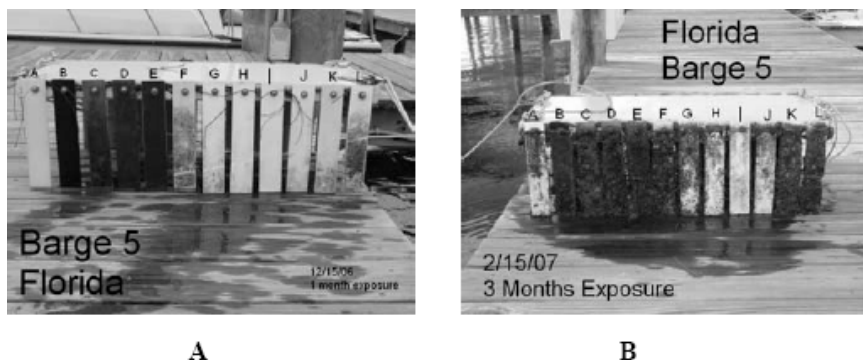
Figure 8: Generation 4 coatings on one side of Barge # 5 tested in Palm Harbor, FL after the (A) 1 month and (B) 3 months exposure. Samples A-D were coated with commercial and control paints. Notice exceptionally good performance of samples H-J from our coating formulations.
